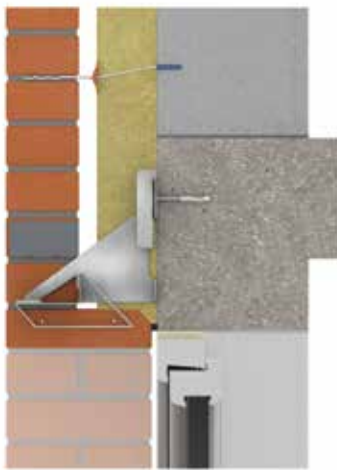
Fig. 29 - NA Masonry Support System
