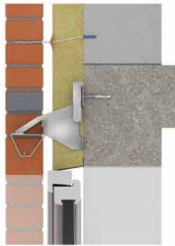
Fig. 27 - NC Masonry Support System
