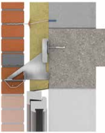
Fig. 26 - NA Masonry Support System
