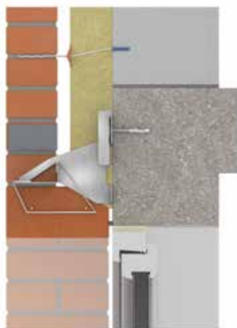
Fig. 30 - NC Masonry Support System
